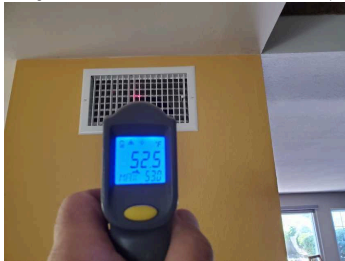
Cooled temperature at register downstairs
