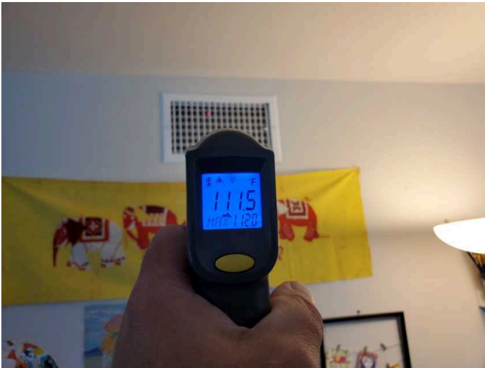
Heated temperature at register in master
