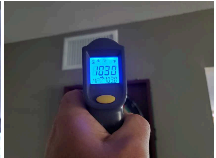
Heated temperature at register downstairs
