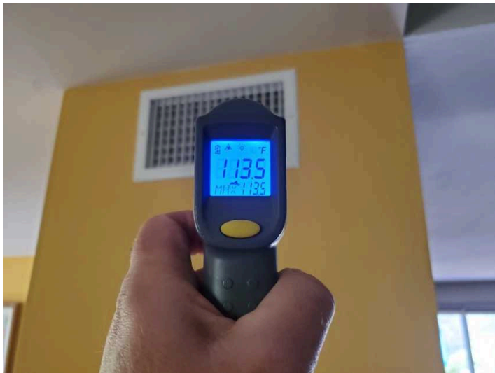
Heated temperature at register downstairs
